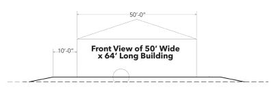
New elevated building dirt pad to provide sufficient drainage away from new building. Elevation of the new building pad will vary per jobsite and condition of surrounding existing grade and/or structures.
